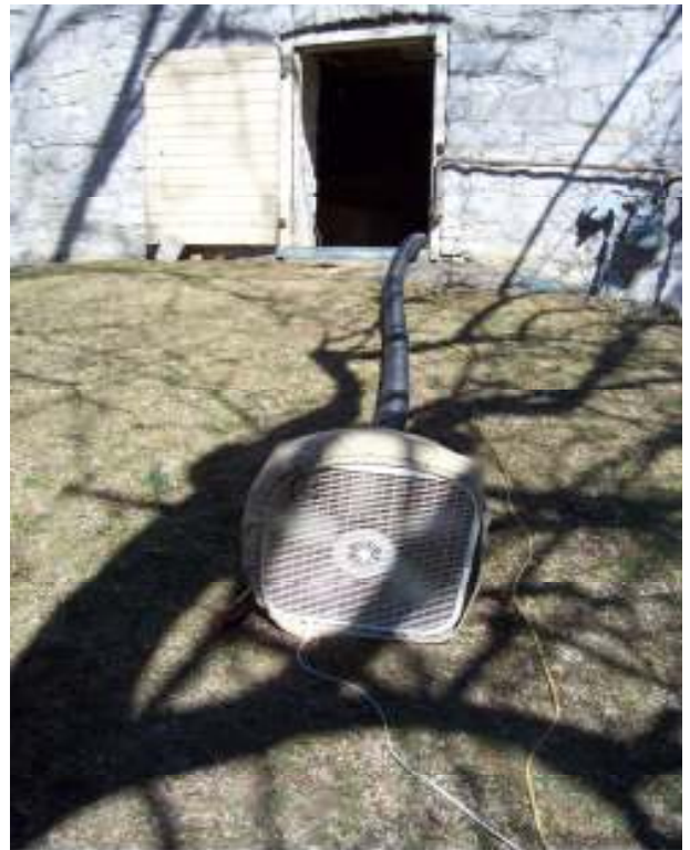
This fan pushes air through the air pipe to our dig site. It has made a big difference.
